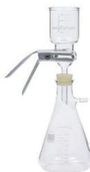
3. Vacuum-filtration apparatus with (from top till bottom) a suspension reservoir, a clamp, a filter holder, a rubber seal and an Erlenmeyer flask with outlet.
