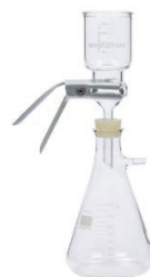
3. Vacuum-filtration apparatus with (from top till bottom) a suspension reservoir, a clamp, a filter holder, a rubber seal and an Erlenmeyer flask with outlet.
