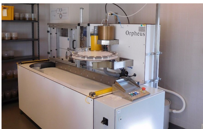
2. AZC, automated zonal centrifuge, is a specialized machine able to isolate approximately 95% of all nematodes from a soil sample (100mL) into a small beaker (40mL nematode suspension).
