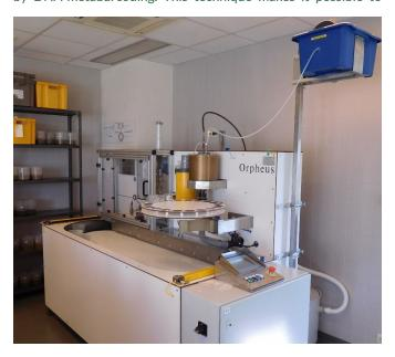
AZC, automated zonal centrifuge, is a specialized machine able to isolate approximately 95% of all nematodes from a soil sample (100mL) into a small beaker (40mL nematode suspension).
