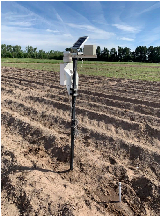
1. A weather station installed on potato crop.
