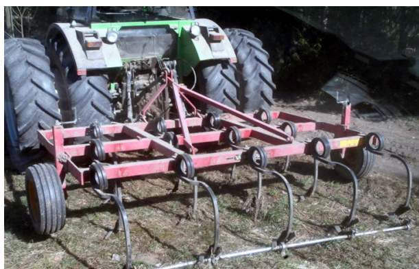
1. A light tillage tool and a lot of wheels result in low stress for the soil.
