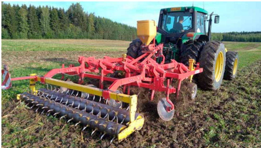
1. Minimum tillage with a sweep-tine cultivator and sowing a cover crop simultaneously in the autumn.
